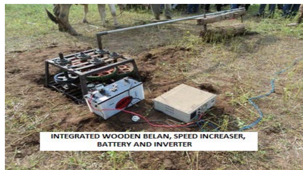
Fig. 1: Integrated Belan, Speed Increaser, belt&pulley, alternator and battery.
